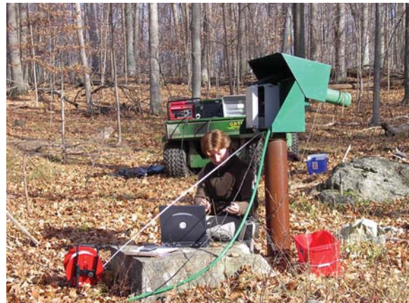
Collecting data from a groundwater monitoring well.
